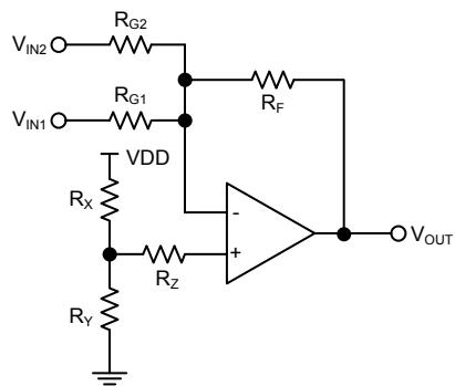
$$R_{VIN-} = \frac{1}{\frac{1}{R_{G1}} + \frac{1}{R_{G2}} + \frac{1}{R_F}}, \quad R_{VIN-} = \text{反相输入的总电阻。}$$
